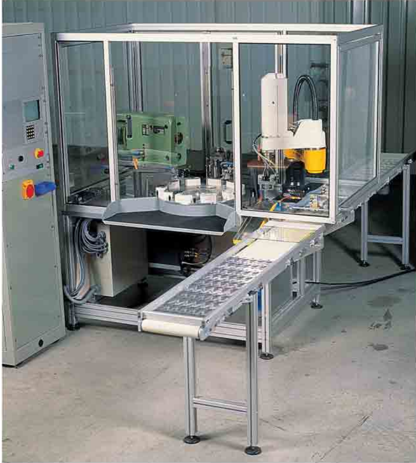
Semi-automatic assembly, inspection and packaging station, with NORCAN frame, housing and conveyor.
