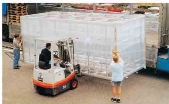
Large machine frame : The judicious use of closed and half closed profiles resulted in a structure of high torsional rigidity allowing shipment of the fully assembled structure.
