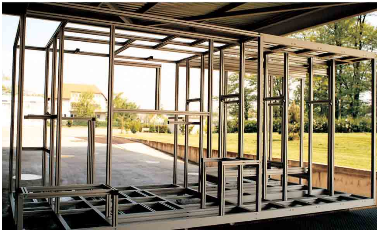
Large machine frame : The judicious use of closed and half closed profiles resulted in a structure of high torsional rigidity allowing shipment of the fully assembled structure.
