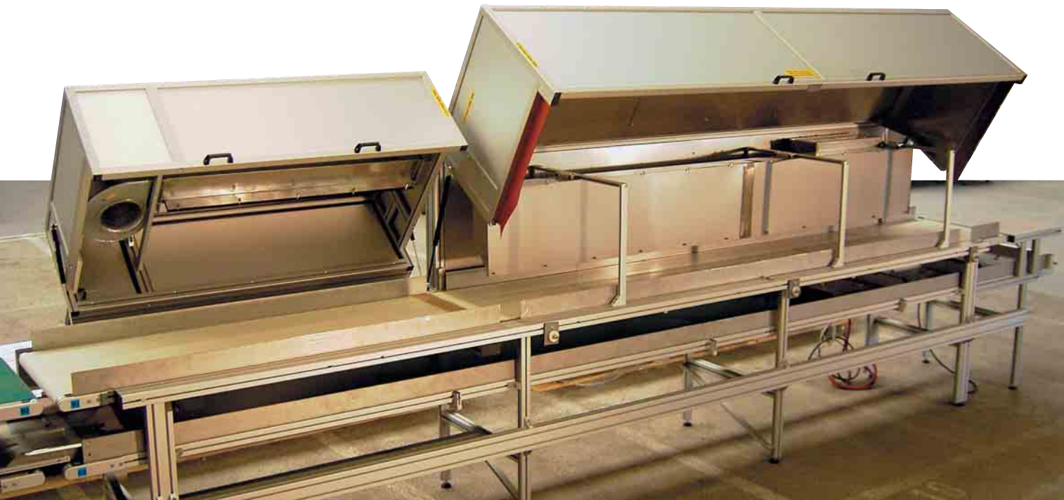
Conveyor line for the drying of ceramic pieces with work station and a pivoting conveyor for the passage of a fork lift truck.
