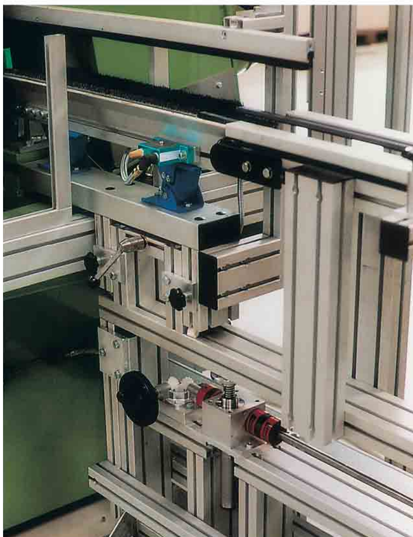
Large machine frame : The judicious use of closed and half closed profiles resulted in a structure of high torsional rigidity allowing shipment of the fully assembled structure.
