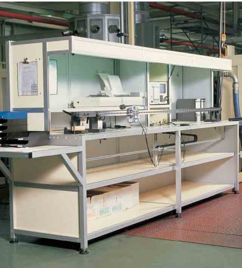
Work station for assembling and the computerised inspection of precision guide rails.
