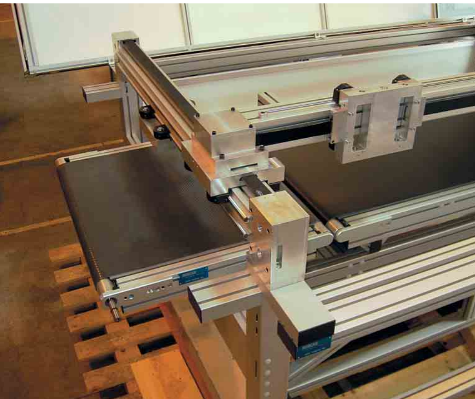
Machine frame with integrated guards, conveyors and an axis xy for very high accelerations.
