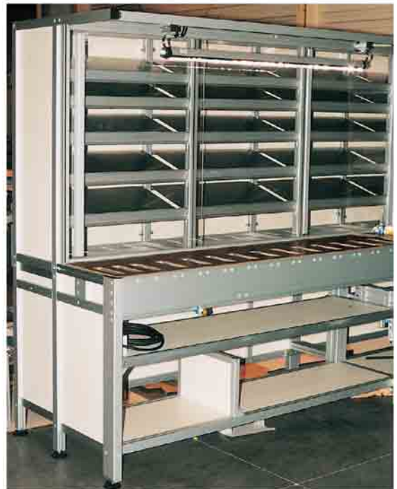
Work station for assembling and the computerised inspection of precision guide rails.
