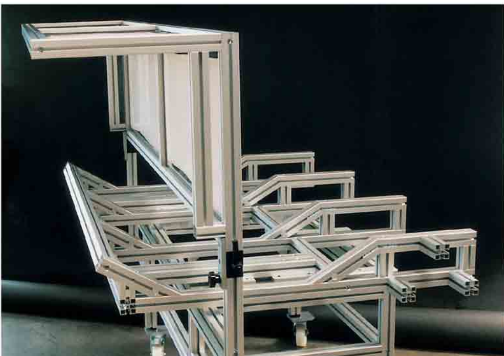
Frames and workstation: The two examples on the top of the page show safety housings incorporated into the machine frame.
