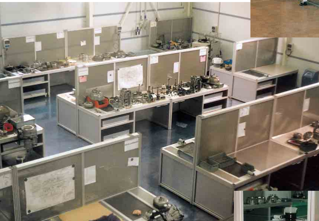
Maintenance and repair shop equipped with NORCAN made to measure work stations. The use of closed and half-closed profiles resulted in structure without visible slots.
